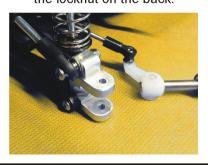
Using the original U brackets, attach them to the wishbones with the 12mm screws, washers and locknuts.
