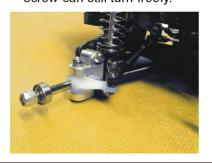
Attach the front hub carriers to the wishbones as shown using the 25mm screws, washers and locknuts.
