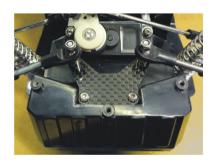
10) Attach the upper links to the hubs with 25mm screws, place a washer between the rod end and hub and the locknut on the back.
