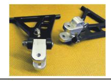
6) Attach the upper links to the carbon plate with the **20mm** screws, spacers and lock nuts as shown.
