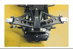
11) Fit the upright to the hub with the 25mm screws, washers and locknuts. Snug these up so the screw can still turn freely.
