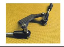
Fit the wishbones back to the bottom of the shocks with the 12mm screws and locknuts.
