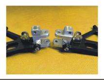
7) Fit the carbon plate to the chassis with **10mm** screws.
