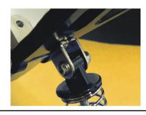
**12)** You may need to wind the steering links out a little to adjust the toe in/out to achieve straight running.
