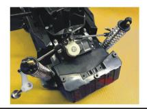
4) Do not over tighten, make sure the screw can still be turned freely.
